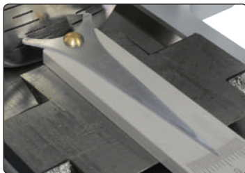
▲ Sliding Apron with built in +5/-5 degree face angle gauge, and a 3" face alignment edge is all that's needed to setup heads correctly prior to measuring lie, loft etc.
