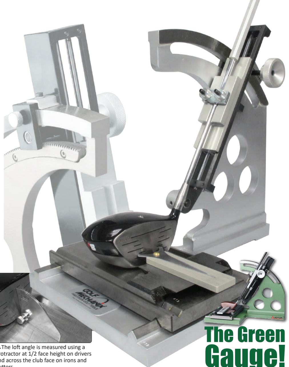
▲ The geared lie angle protractor provides smooth and precise controls matched to the Vernier style lie angle scale, having a resolution of 1/10 of a degree.
