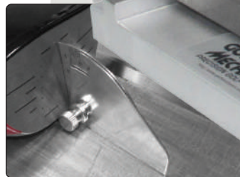
▲ The loft angle is measured using a protractor at 1/2 face height on drivers and across the club face on irons and putters.
