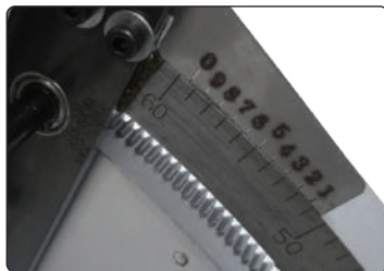
▲ The geared lie angle protractor provides smooth and precise controls matched to the Vernier style lie angle scale, having a resolution of 1/10 of a degree.
