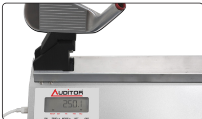
▲ Components are weighed on top of the grip stop to 1 gram precision
