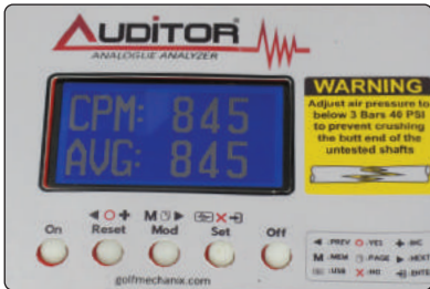
▲ New Shaft frequency analysis engine. Has auto reset and auto averaging function and Programmable profiling zones.
