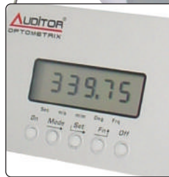
▲ Decimal unit display with averaging function for last 5 measurements
