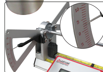
▲ Redundant torque scale for cross checking the digital readout.
