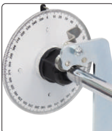
▲ Adjustable deflection height at the fulcrum for load induced shaft spine auto rotation.
