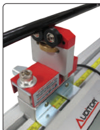
▲ Adjustable deflection height at the fulcrum for load induced shaft spine auto rotation.
