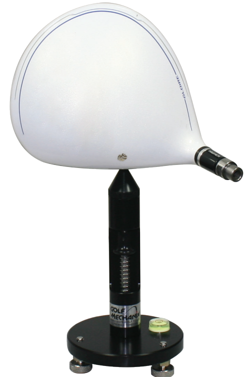
The Classic Plus model adds to the design levelling feet and bubble level for added precision
