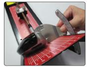
▲ Clubhead soling plate provides precise postioning for measuring lie and loft angle as well as face procgression on woods, irons and putters
