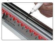
▲ Set the butt trimming gauge to the desired playing length for the driver or lead iron, pre-assemble the club and adjust for lie before transferring butt trim to shafts
