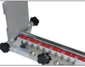
▲ Set the gauge at the desired tipping increment for the driver or lead iron, and mark the shafts one at a time using the guide.
