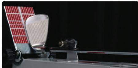
▲ Soling plate slides forward to adjust for club length automatically while improving grip, shaft and head sight line.
