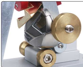
▲ Triangulated high stability isostatic clamping arrangement with conical soling rollers support sole at both ends to secure iron in position.
