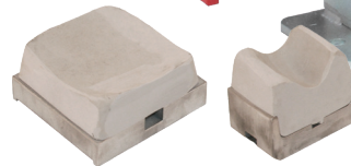
▲ Molded pads lifted of a typical driver. The pads then used to cradle the head when bending
