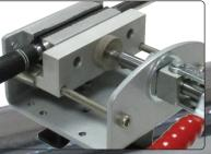
A Quick vise clamp with round jaws does a good job at securing shafts at or near the butt end of the shaft, like when gripping.
