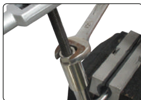
▲ Tighten the nut after heating the hosel to soften the epoxy
