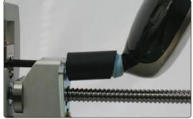
The spacer is rigid enough to push against the hosel when removing shafts.
