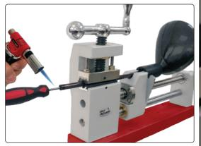
▲ The kit also includes a skewer for heating up the hosel from the inside of the broken shaft.
