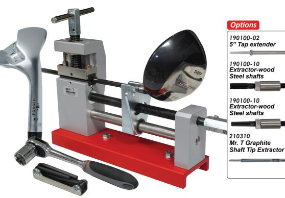
The jack screw assembly comprises the carbonitrated high thread count with ball bearings\* at each end, The jack nut fitted with a low friction DRYMET flanged bushing, the linear guide rod, hosel gate and power spring.
