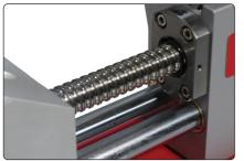
▲ Linear ball screw and twin guide rod assembly
