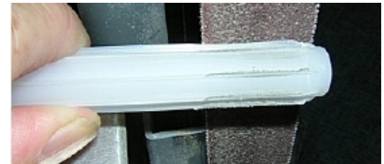
Reduce the O.D of the insert by sanding down the ribs.
